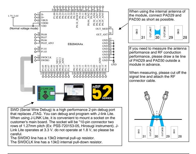
The bypass capacitor necessary for the power supply line is installed inside the module. So you do not need to add external capacitors. However, in case of the operation with the battery, we recommend that you add a bypass capacitor about 100uF in view of the voltage drop during TX/RX. Please consider whether it is necessary according to the performance of the customer's battery.
